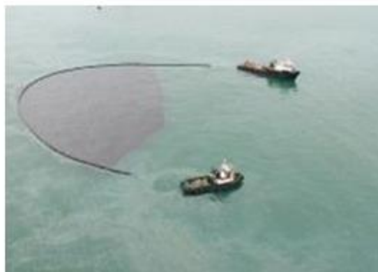
Figure 6.5: Water bourne containment and recovery configurations utilising a single vessel system
