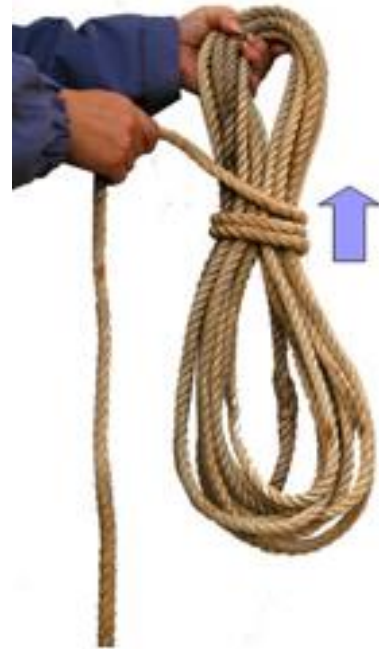
The trick to coiling rope is to twist each loop until the line lays flat
