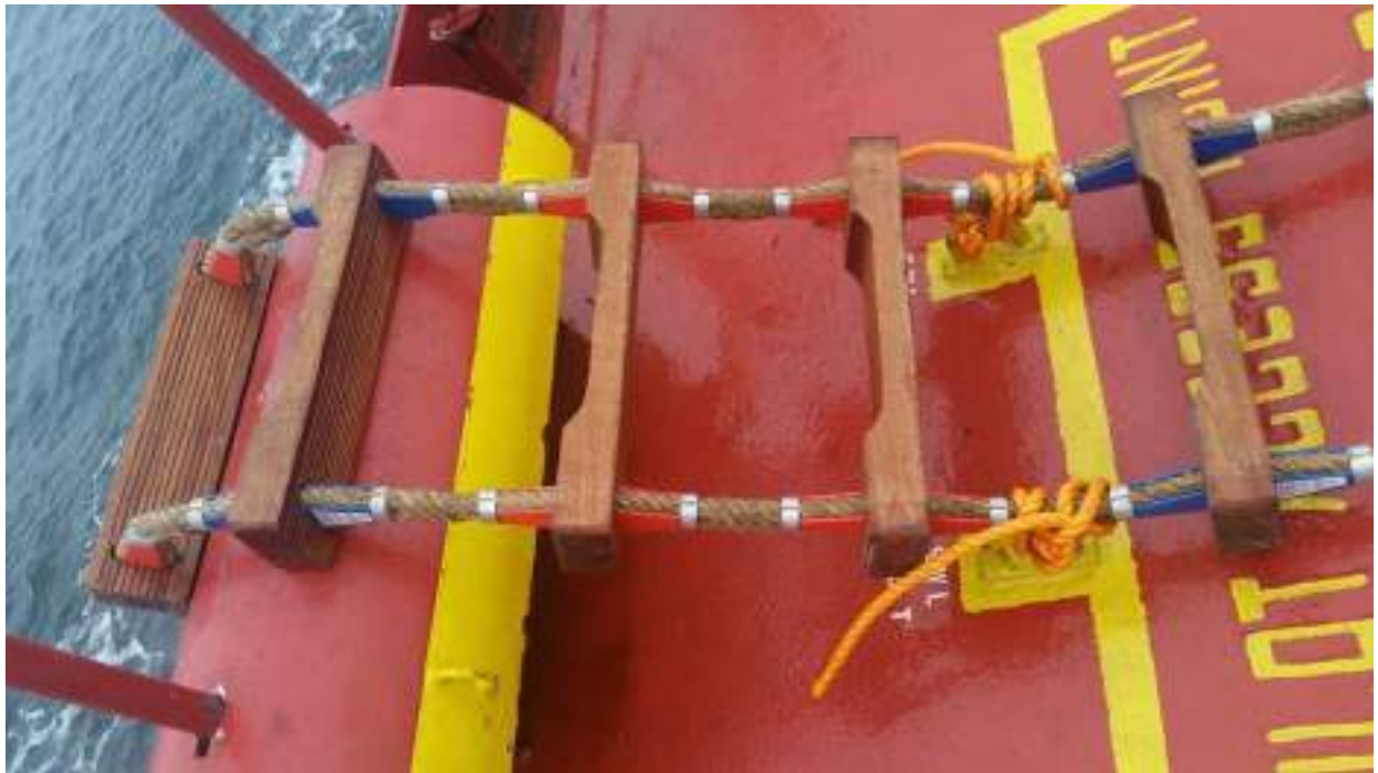
The above shows a correct secondary securing method for a ladder coming off a winch reel.
