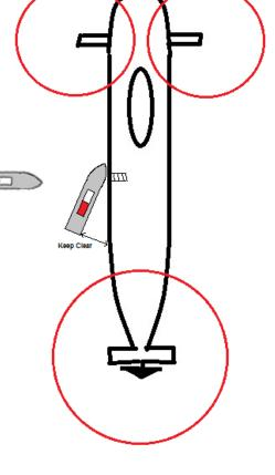
*Note*-Pilot vessels with stabiliser fins outboard to the props and rudders which could easily be damaged by a submarines hull should not generally be used.
