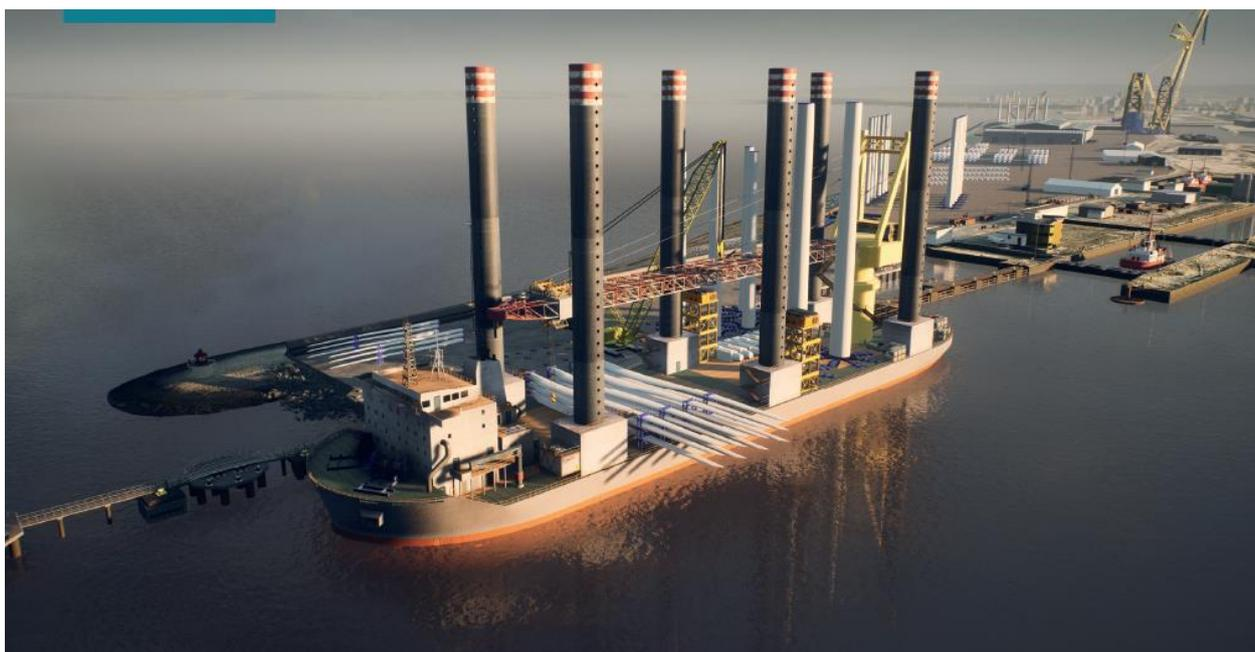
Figure 3-3 Example loading of offshore renewables vessel when berthed and laydown area
