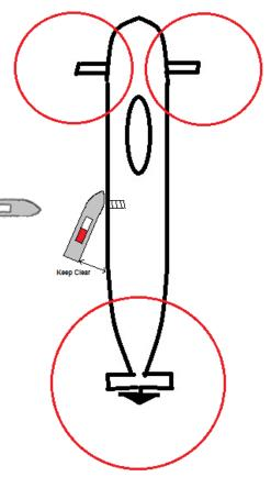
*Note*-Pilot vessels with stabiliser fins outboard to the props and rudders which could easily be damaged by a submarines hull should not generally be used.
