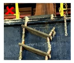
Pilot Ladders should always be rigged with a form of edge protection to stop the ropes from chafing. An Arrangement such as a rounded bar, permanently fixed at the embarkation point should be in place.
