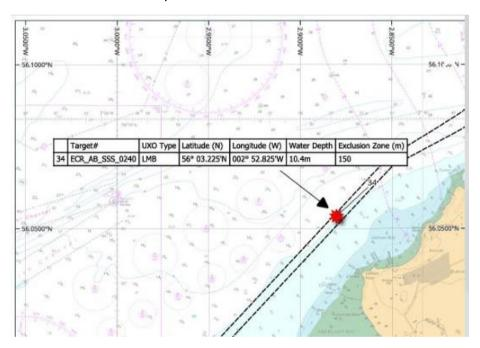
Inch Cape cUXO disposal campaign shall commence on or around the 30<sup>th</sup> May 2025 within the Inch Cape export cable corridor on the cUXO's detailed in the below table:
