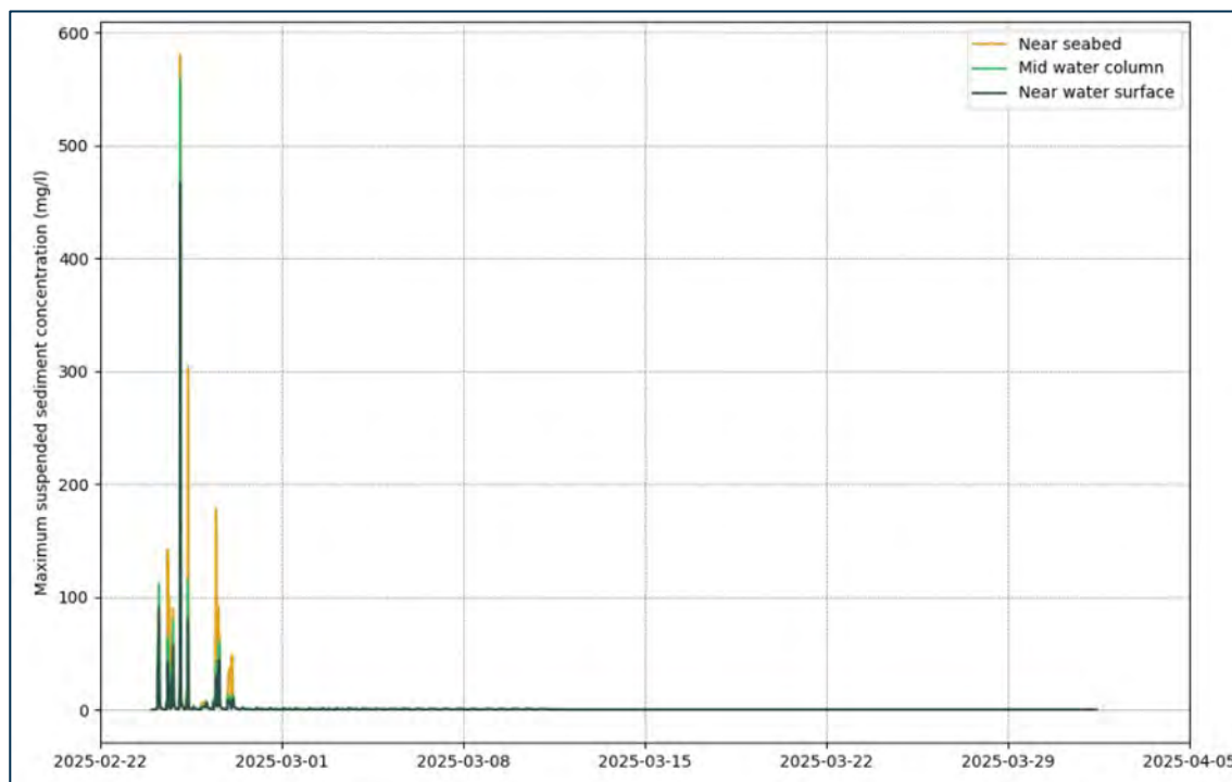
Figure 7-26 Time series of predicted suspended sediment concentrations at the Port of Dundee during dredging for plumes near the bed of the Firth of Tay, mid water column, and near the water surface
