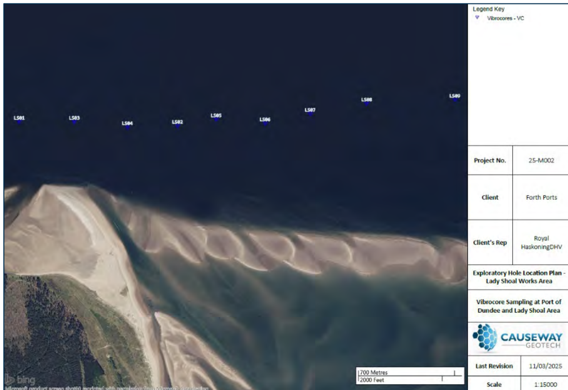
Figure 7-18 Location of vibrocores at Lady Shoal approach channel collected in February 2025
