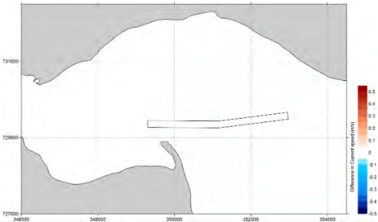
Figure 5-49 Difference in current speed (in metres per second) between 'Existing' and 'Option' during neap tide at the Lady Shoal approach channel 2 (positive means increase of current speed by option and vice versa) – peak ebb
