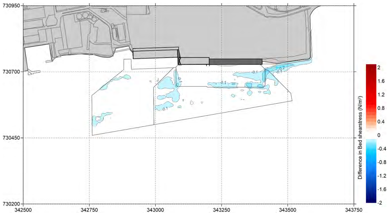
Figure 5-78 Difference in Bed shear stress ( \text{N/m}^2 ) between 'Existing' and 'Option' during neap tide at the Port of Dundee area (positive means increase of Bed shear stress by option and vice versa) – peak flood
