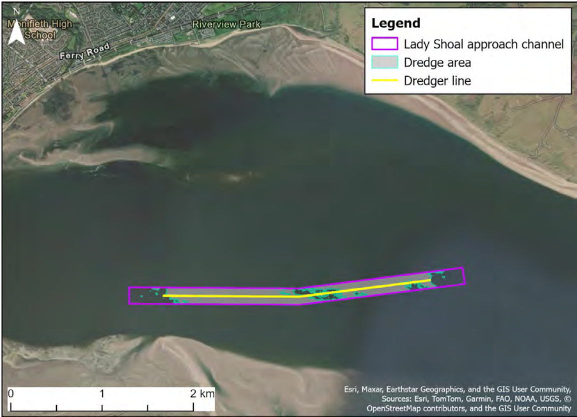
Figure 6-2 Dredger line at Lady Shoal approach channel
