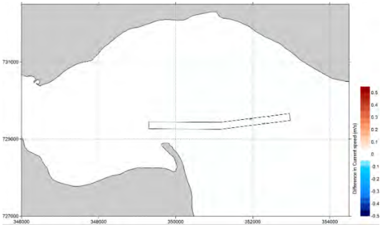
Figure 5-45 Difference in current speed (in metres per second) between 'Existing' and 'Option' during spring tide at the Lady Shoal approach channel (positive means increase of current speed by option and vice versa) – peak ebb
